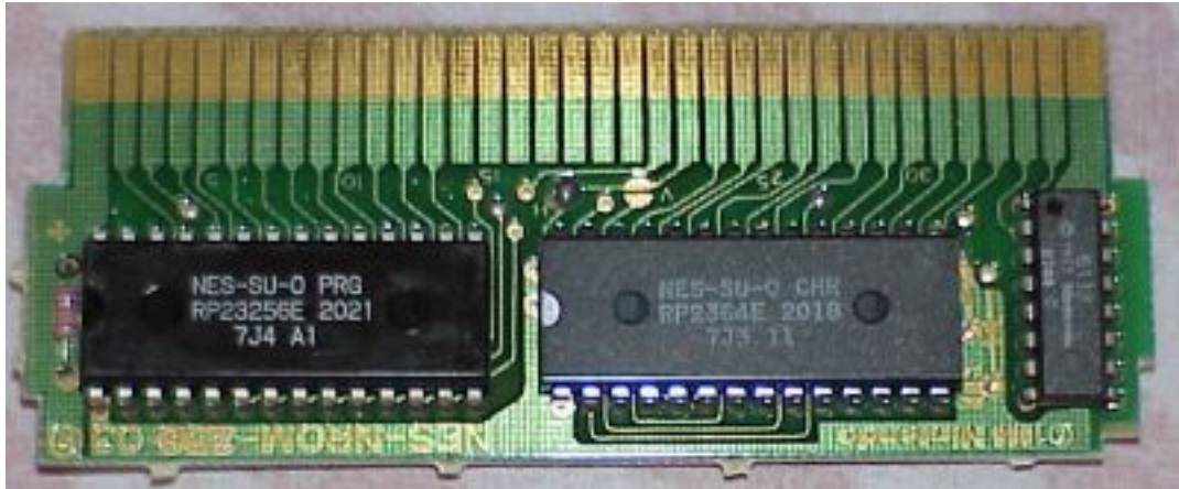
Figure 2.8: The bare PCB of the SMB Cartridge
